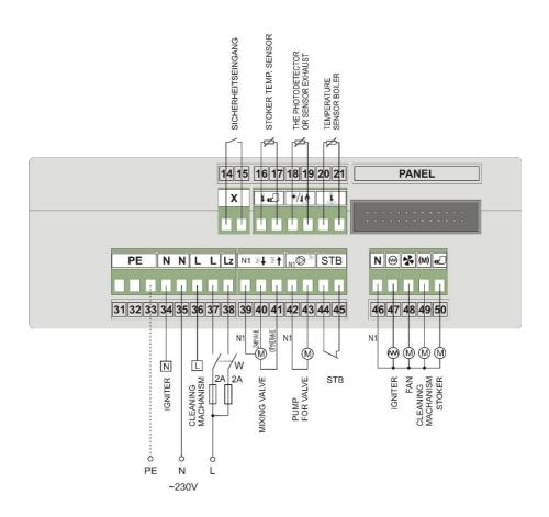
Figure 3. RK-2006SPGM+MZL Controller connection diagram.
