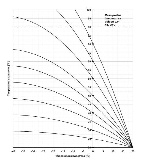
The ratio of weather charcteristics inclination – the parameter defines the CH water temperature, when the outside temperature is 0. The relation between the outside temperature and the CH circulation water temperature for ten exemplary settings of the parameter is shown in the graph.
