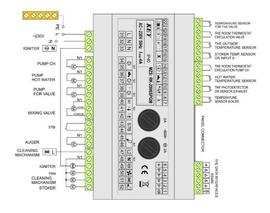
Figure 2. RK-2006SPGM+MZS Controller connection diagram.
