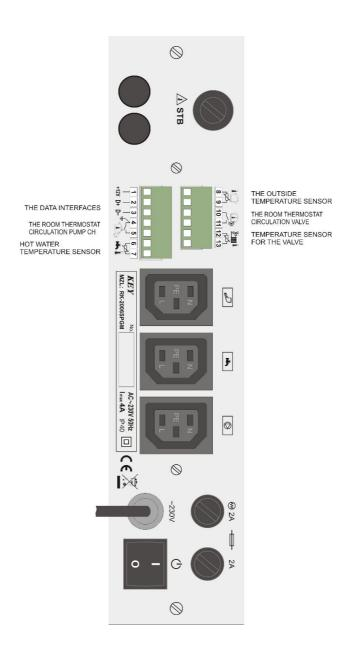
Figure 4. RK-2006SPGM+MZL Controller connection diagram.
