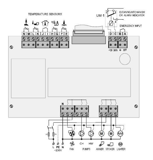
Figure 2. RK-2006LSP Controller connection diagram.
