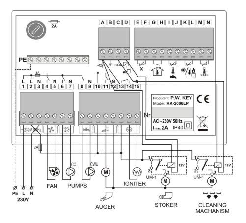
Figure 2. RK-2006LP Controller connection diagram.
